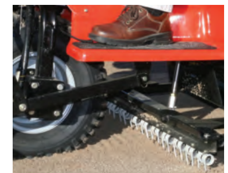
Sand Cultivator, stainless steel
