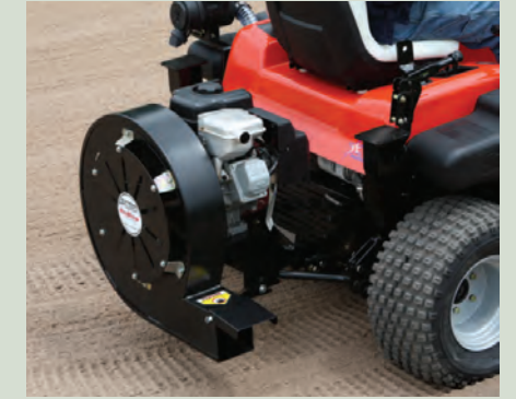
Engine-Powered Leaf and Debris Blower
