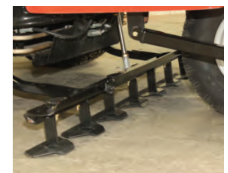
Sand Cultivator triangle-shaped blades
